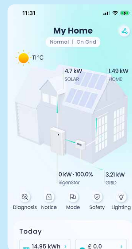
Picture 1 shows a sunny day with the panels generating 4.7kW of power. The battery is fully charged to power the house in the evening. From the power generated 1.49 kw is supplying household needs with the rest sold to the Grid.
